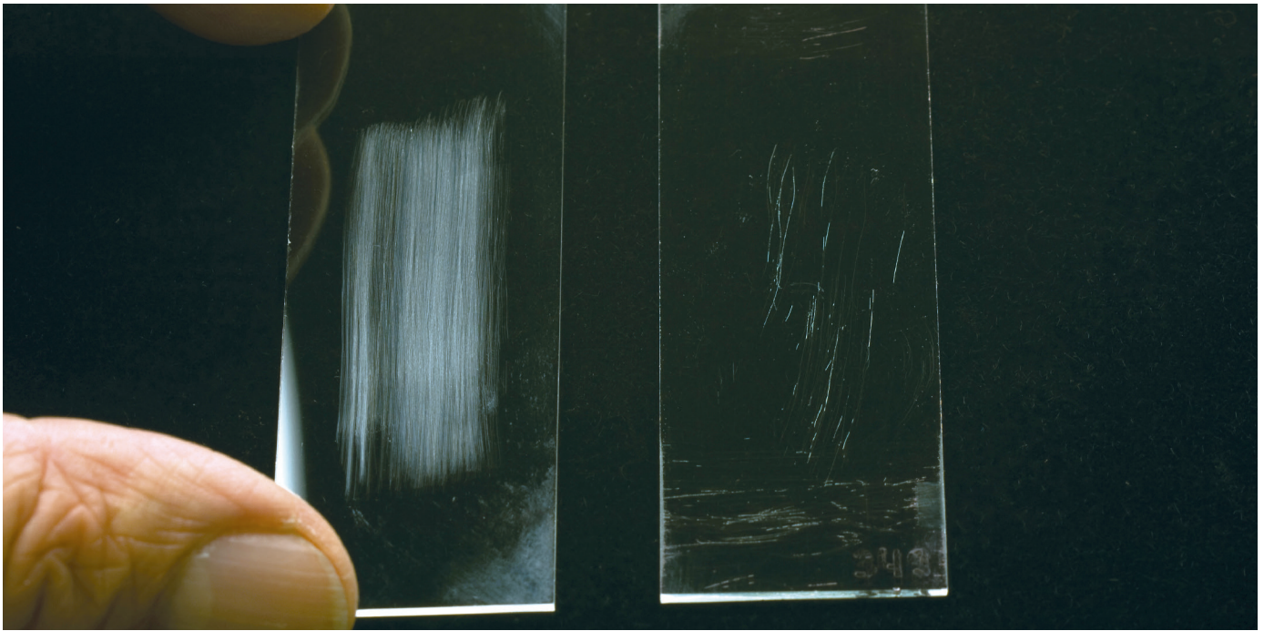
left: glass plates are readily scratched by sandpaper, right: coated glass plates show scratches only after prolonged scratching due to subsurface damages in the glass
